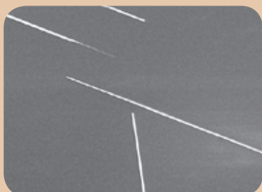
Fig. 2: 50 nm thick WO x nanorods.
